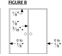
\* Allow extra clearance as required per astragal manufacturer. Certain door and frame conditions may require an extra 1/32"-1/16" clearance. Excessive clearance on fire rated assemblies may violate the requirements of NFPA 80.
