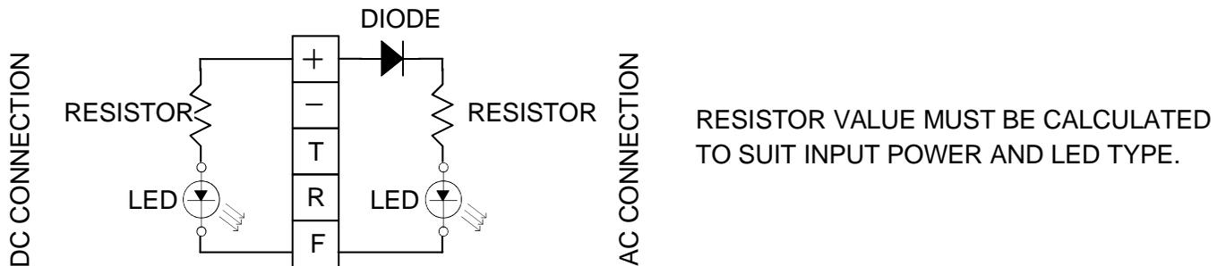
IF THE TIMEMASTER IS POWERED FROM A DC SOURCE, USE THE CONNECTIONS SHOWN AT THE LEFT. IF IT'S POWERED FROM AN AC SOURCE, A DIODE MUST BE ADDED AS SHOWN ON THE RIGHT.
