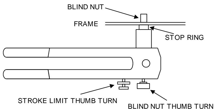
Next note that the stroke limit thumb turn and connecting shaft is present to stop the handles from coming too close when you squeeze the tool and therefore injuring your fingers. It requires no adjustment. Make sure that the handles open and close easily and then thread a
