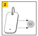
Replace 3-volt (CR2032) battery<sup>1</sup>, observing polarity, and reassemble.
