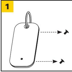
Remove back screws (2) and disassemble.
