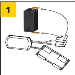
Connect transmitter<sup>1</sup> to push plate (NO and COM) and insert into box.
