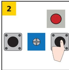
Press and release desired learn button (red LED on receiver will illuminate)<sup>1</sup>.
