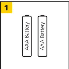
Replace 2 AAA batteries observing polarity.
