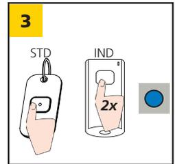
Press transmitter TWICE (blue LED on receiver will illuminate).
