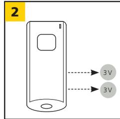
Replace two 3-volt (CR2032) batteries<sup>1</sup>, observing polarity, and reassemble.
