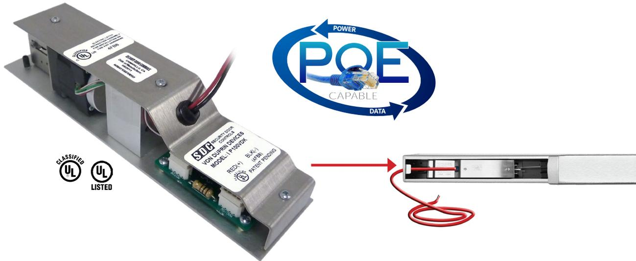
The SDC IP100 Series 12V PoE-Capable Electric Latch Retraction Kit enables electric access control and dogging of mechanical exit devices. When energized the motor retracts the exit device latch and pulls the pushpad\* into the dogged (depressed) position enabling momentary or sustained push and pull operation of the door.
