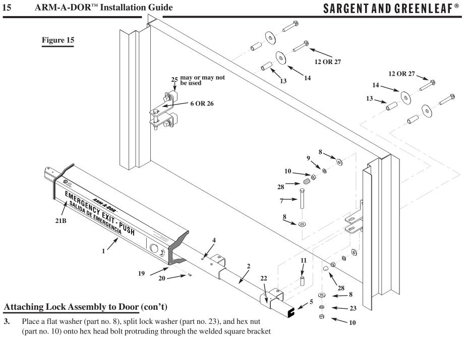
and door bracket. Hand tighten leaving hardware loose enough to adjust lock position.
