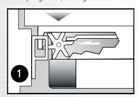
2. When push bar is depressed, the deadlocking slide moves back, allowing the door to unlock from the strike. This unique interlock provides solid security and prevents jamb spreading.
